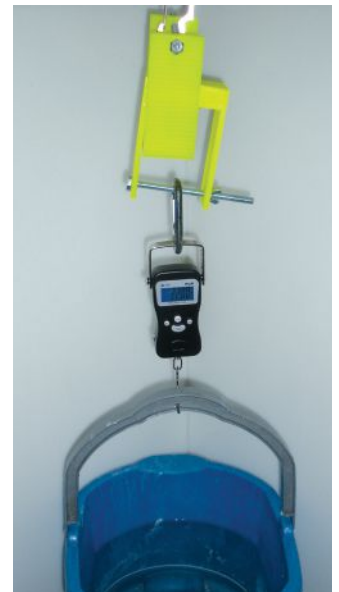
Crush test setup, post-crush.
